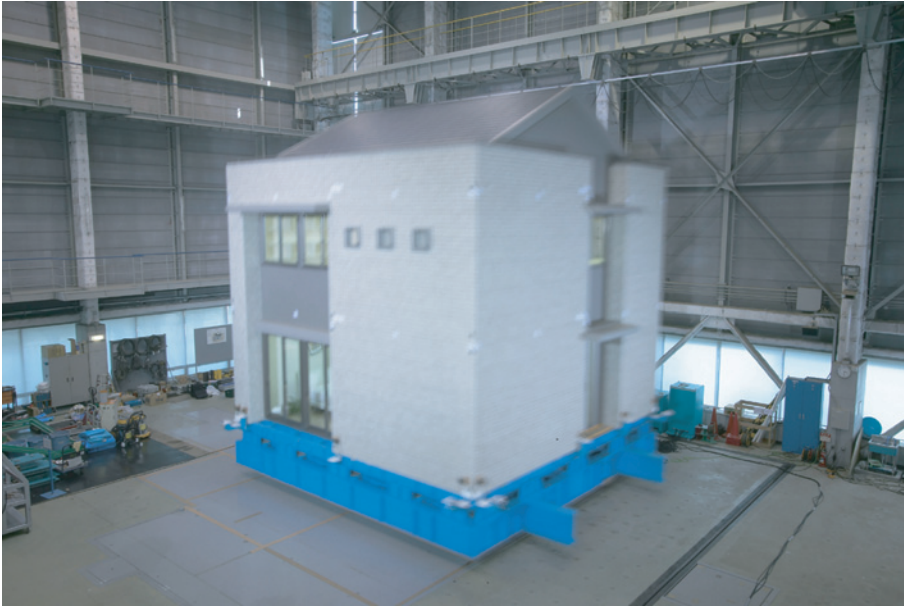
CS 7.10. Full-scale MGeo seismic tests.
