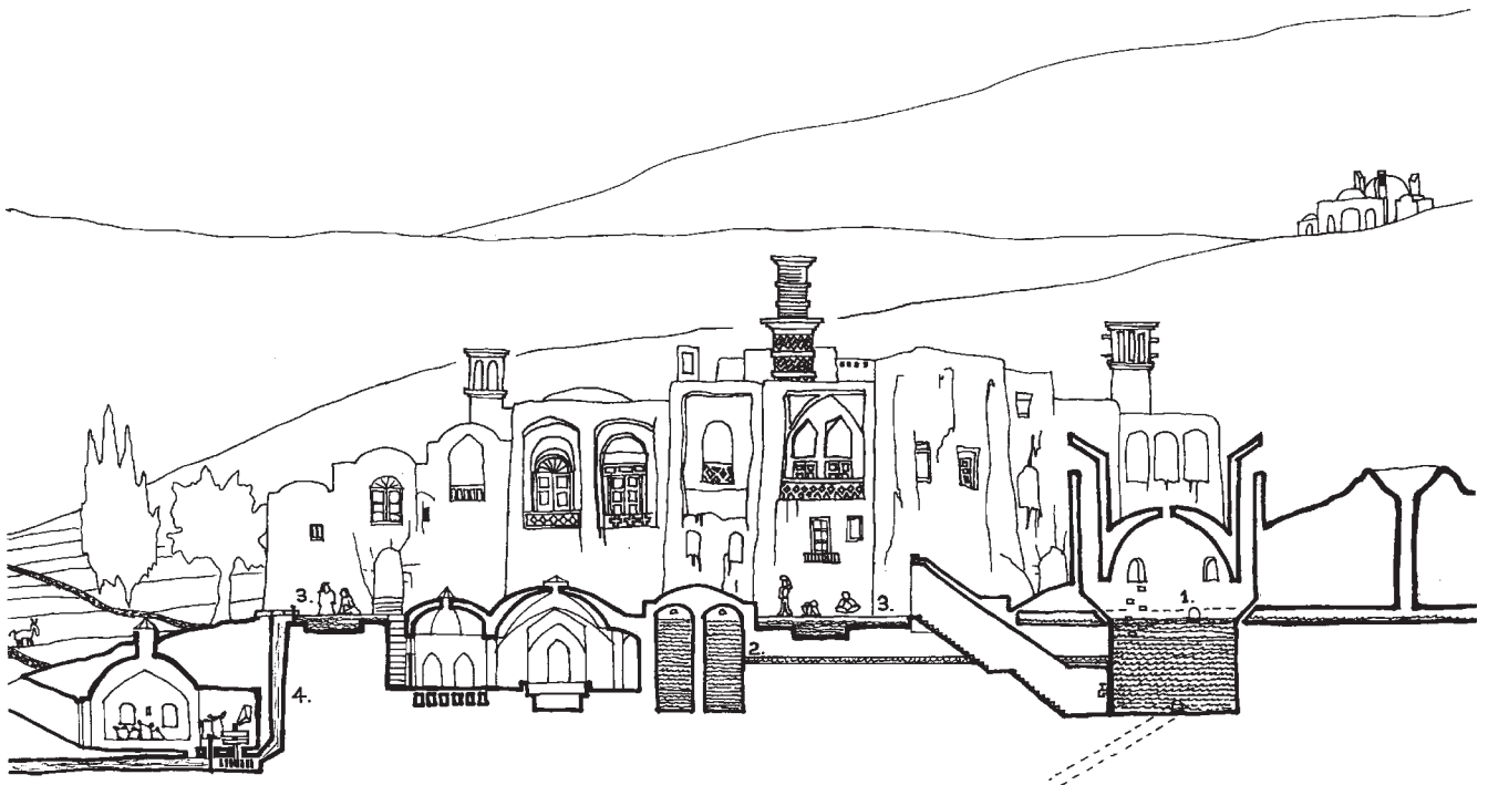
10.5. Section through the village of Khoranaq, in the Central Persian desert north of Yazd, showing the passage of the water from an underground channel or Qanat through the village, being used from clean to dirty uses. On its path the underground stream is used to: 1. fill the drinking water cistern; and 2. the bath house or Hammam; where it emerges it is used for 3. washing of kitchen ware and clothes (without detergents); and 4. drops down a vertical chute to turn the horizontal mill wheel and emerges again to provide drinking water for the animals and water for the fields. Washing of clothes with detergent is done downstream of the animal drinking water pond and the water run to waste (Roaf).
